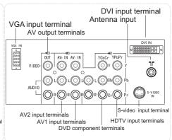
S-video input terminal: Special video (S-VIDEO) AUDIO: L/MONO Track (L/MONO), R Track (R) AV output terminals: VIDEO AUDIO: L/MONO Track (L/MONO), R Track (R) AV2 input terminals (MONITOR): VIDEO AUDIO: L/MONO Track (L/MONO), R Track (R) Av1 input terminals (MONITOR): VIDEO AUDIO: L/MONO Track (L/MONO), R Track (R) DVD component terminals:
